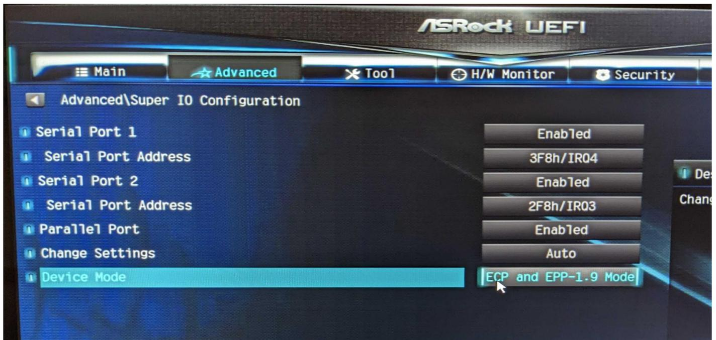
Make sure the parallel port is enabled, and that it's in ECP+EPP mode. The version of this mode doesn't really matter! (mine has 1.9 and 1.7)
